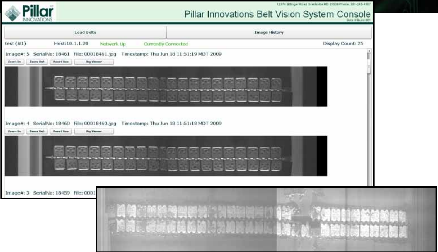
Actual Captured Splice Image
